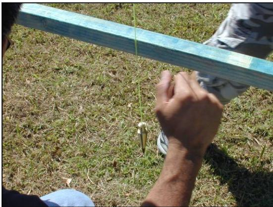
A-frame legs on contour, plumb line aligns with notch
