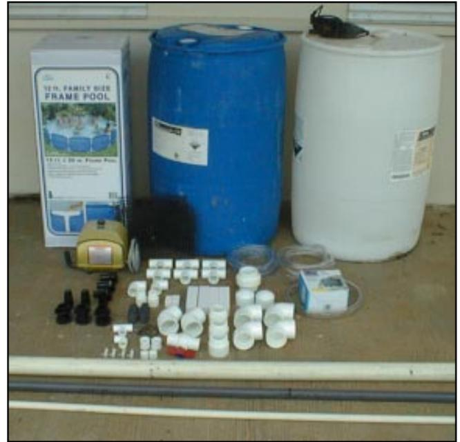
Parts used in the recirculating aquaculture system, including pool, plastic barrels for filtration tanks, air stones, pvc pipes and fittings, water pump and air pump
