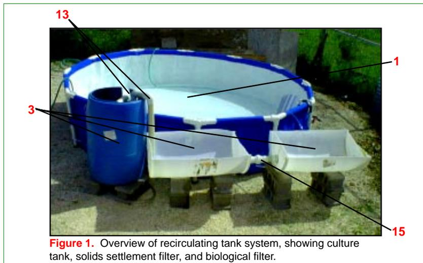
Figure 1. Overview of recirculating tank system, showing culture tank, solids settlement filter, and biological filter.
