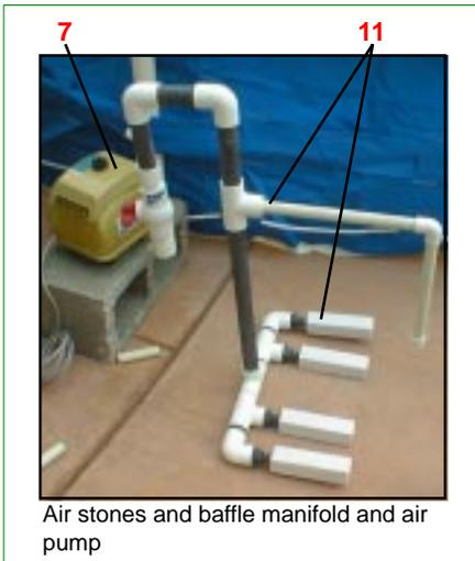
Air stones and baffle manifold and air pump
