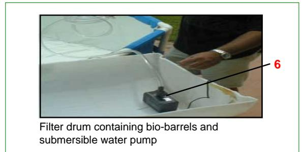
Filter drum containing bio-barrels and submersible water pump
